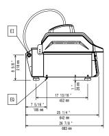
Electrical inlet (power) Electrical Outlet
